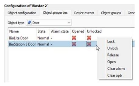
Control of the individual object can be selected by right-clicking the mouse over the object for which control is required.
